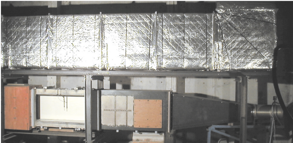
Fig. 1. The ISVR progressive wave tube facility.
