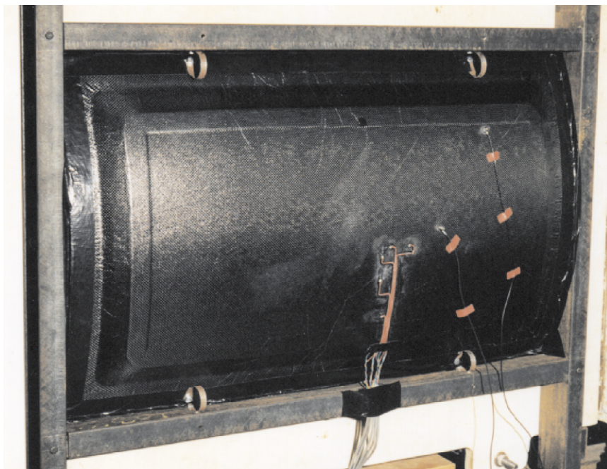
Fig. 6. Panel 3 secured in the PWT aperture using four circular steel springs.
